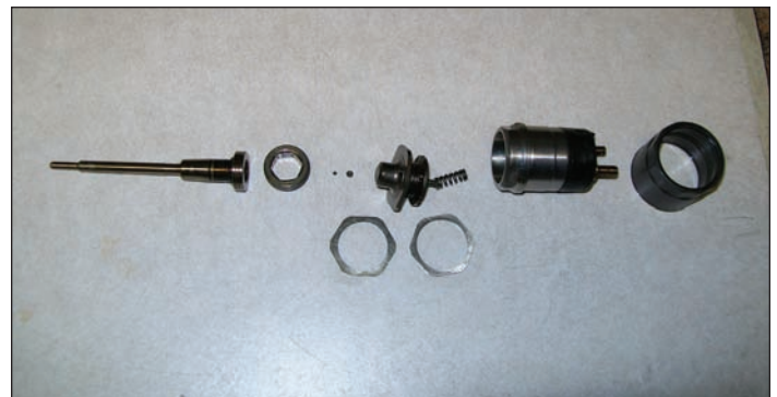
72i17 Disassembled top half of HPCR injector.
