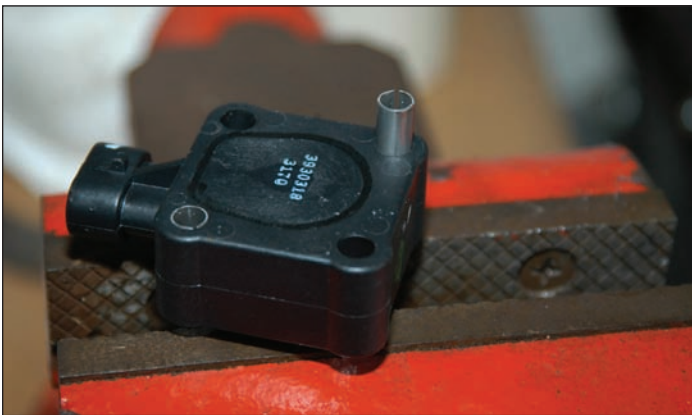
Remove the two steel sleeves from the TPS.
