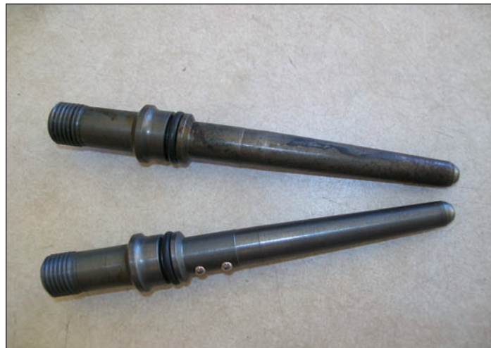
72i13 Rust pitted connector tube above a good tube.
