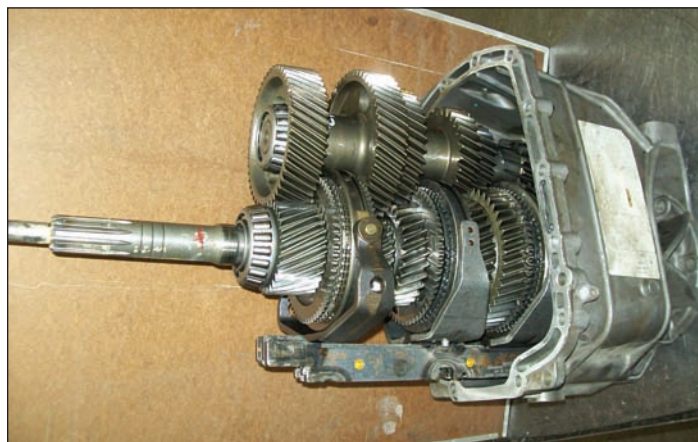
71-24 Rear half of the case with mainshaft and cluster assemblies.
