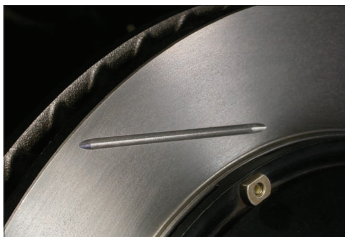
A typical rotor before bed-in. Note the clearly defined machining marks on the rotor face.
