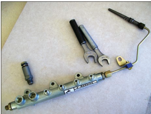
72i4 The high pressure fuel rail with the pressure relief valve above it on the left. In the center are the shortened wrenches used to remove the #6 fuel line while clearing the cowl of the truck. The #6 line is threaded into the rail and an injector connector tube.
