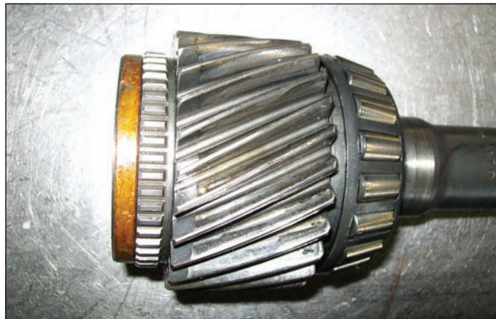
71-18 Input with wear indicating misalignment of gears.
