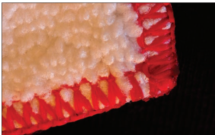
Figure 4: Griot's white wax-removing cloth has a well-controlled edge weave, and did not shed any fibers. There is a melted portion to keep things from unraveling but it is tightly contained.
