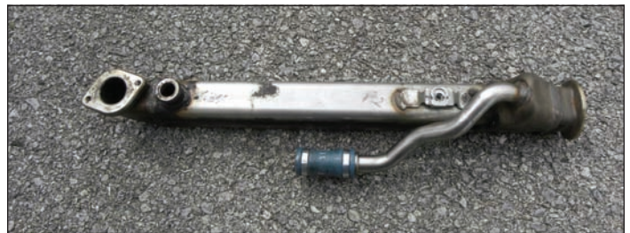
EGR cooler. Coolant enters and exits through round ports while exhaust gases enter and exit at ends.
