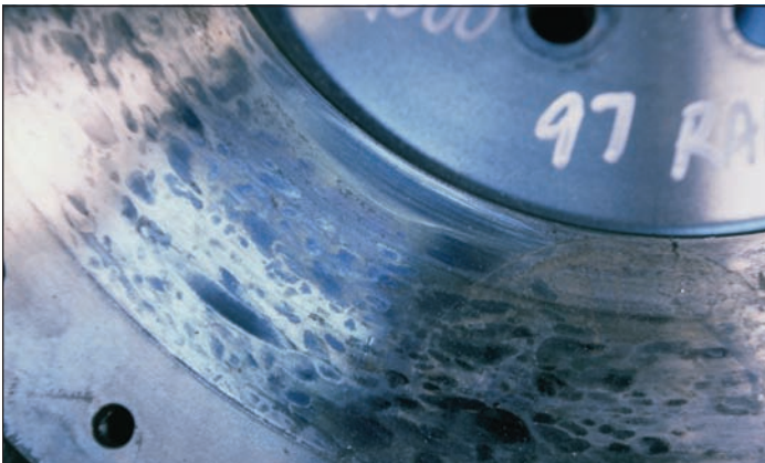
Shown is a used flywheel that needs resurfacing or replacement.
