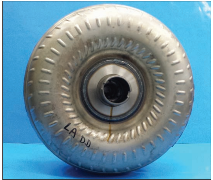
The one-way clutch of the AS68RC was eliminated to cut costs, complexity, and make room for the new automatic's larger torque converter in the same overall length. The new converter carries about half the transmission's ATF capacity and it must be able to slide on the input and stator splines during shifts.
