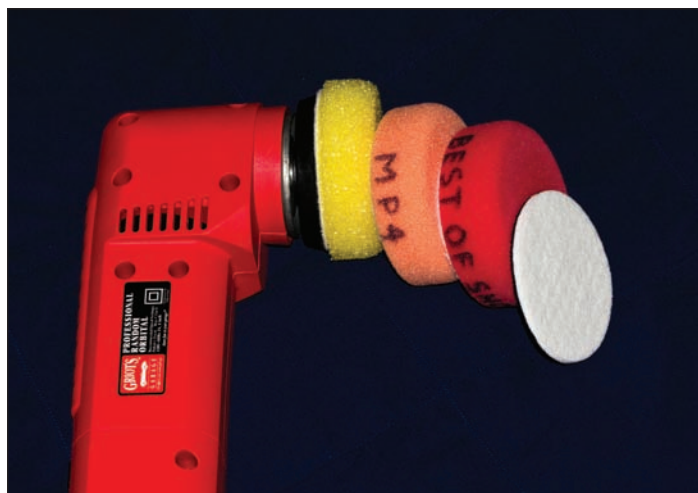
Figure 13. Griot's 3" random orbital with a versatile collection of pads. From left to right: yellow scrubbing pad (installed), orange polishing pad dedicated to "machine polish 4", red waxing pad dedicated to "best of show" wax, and finally the white, glass polishing pad.
