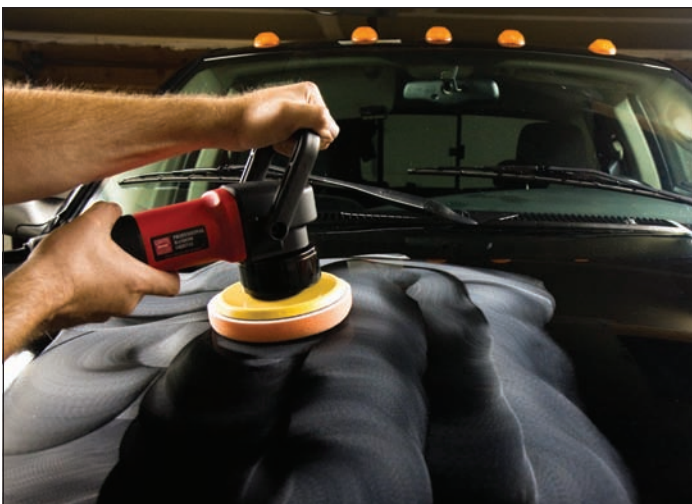
Figure 6. Machine polishing with Griot' orange polishing pad and “Machine Polish 3”.
