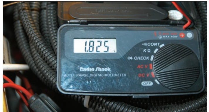
I now have 1.8 volts at the "idle" position of the TPS.
