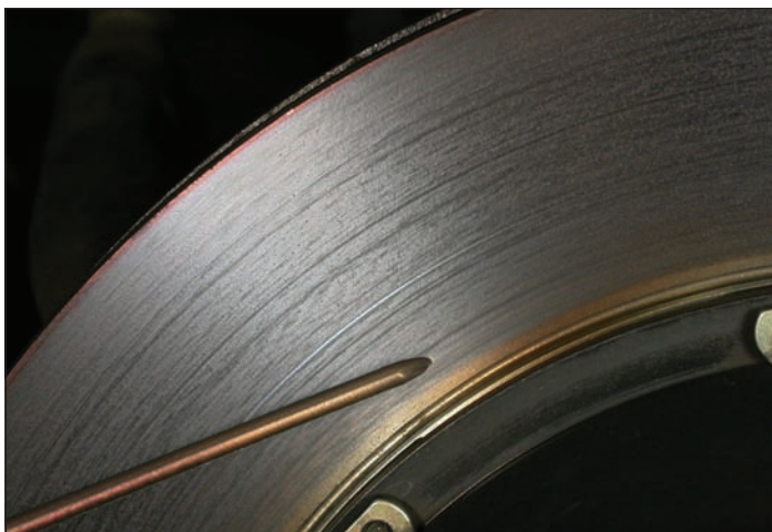
A typical rotor after bed-in. The soft gray haze on the rotor face is the transfer layer material.
