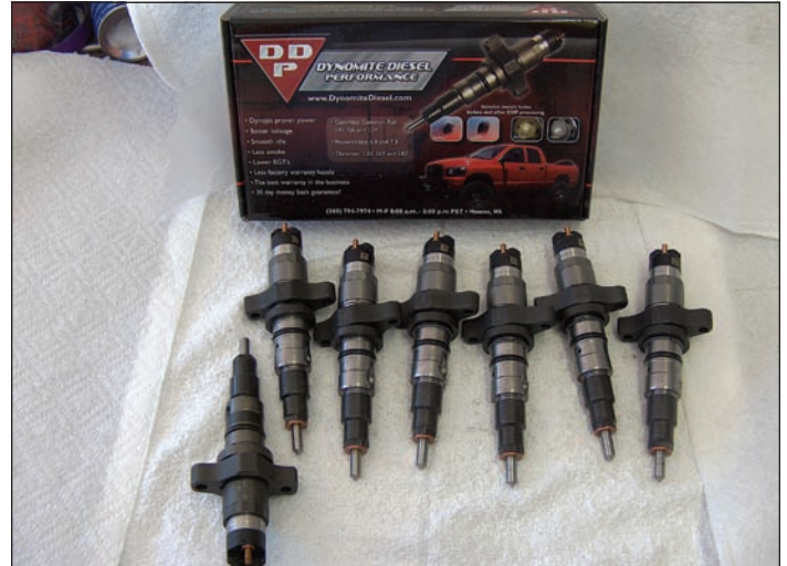
72i11 Six new DDP Stage 1 injectors with the new Bosch shiny white coated steel bodies. Facing the other way is a used injector with the regular gray colored steel body.
