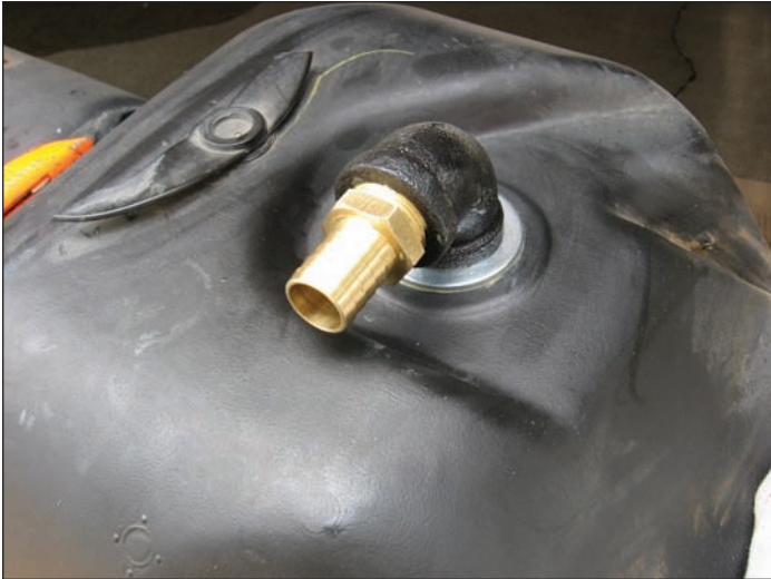
The main-tank pickup tube is installed in a raised boss almost as if designed for my use. The steel elbow and nipple terminate in the tank with a 3/4" PVC drawtube that drops straight down to the bottom of the tank, allowing fuel to be pumped into the upper tank when needed. The tank was dropped to install this O-ring-sealed connection.
