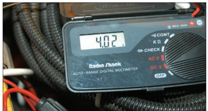
Manually moving the TPS from idle to WOT the voltage displays smoothly to 4 volts.
