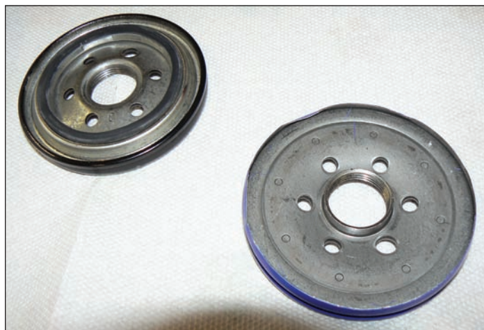
Note the small 1/4" holes in the Mobil and STP base plates.
