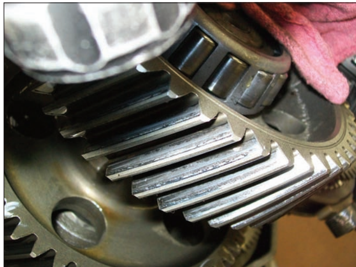
71-29 Electrolytic pitting of gear teeth.
