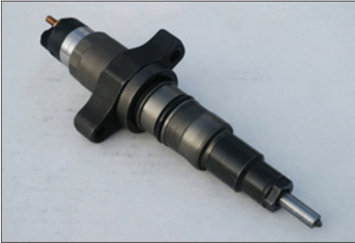
72i3 Bosch injector for the HPCR system. The extra height of the injector for the new common rail system, compared to older style mechanical injectors, accommodates the electrical control mechanism to open and close the injector. Prior designs on our Turbo Diesels used fuel pressure to open and close the injector.
