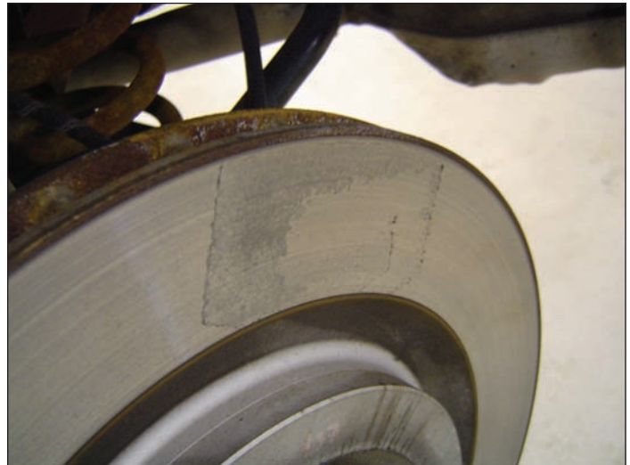
Pad printing is due to corrosion while parked. This is classic TV in the making, and pulsation is only a few miles away.
