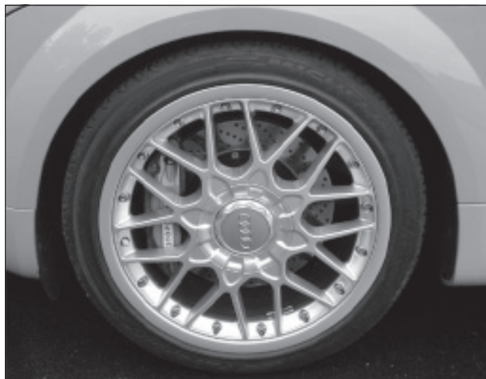
Figure 7 – Filling the wheel with brake hardware
