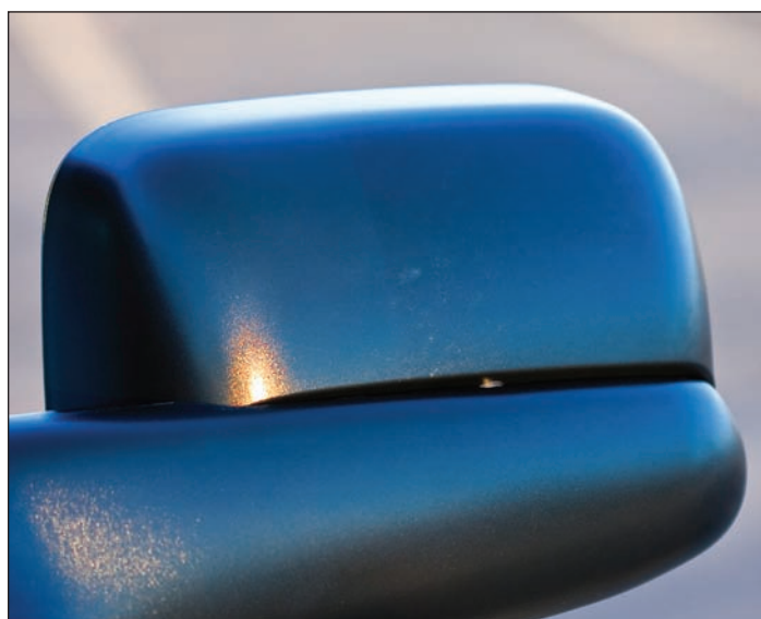
Figure 12: Rearview mirror after using Griot's 3" random orbital fitted with the yellow scrubbing pad (left side). The right side was cleaned with the same pad, only by hand.
