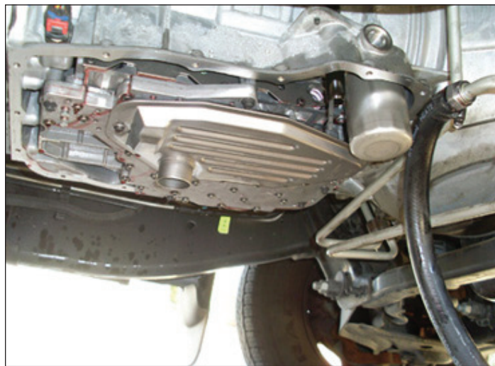
The bottom cooler line is the return-to-transmission line. Remove it with a 1" open end wrench. Clamp a 3/4" ID hose over the threaded barb and direct the fluid into a 5-gallon bucket.
