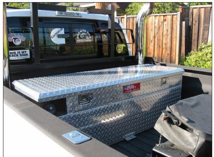
The tank-toolbox combinations offer accessory as well as fuel storage in a compact unit. Even placed farther back in the bed to accommodate the exhaust stacks, this diamond-plate model still sits well ahead of the fifth-wheel hitch and is installed using the weld-on tabs to bolt to the truck bed for a secure installation.
