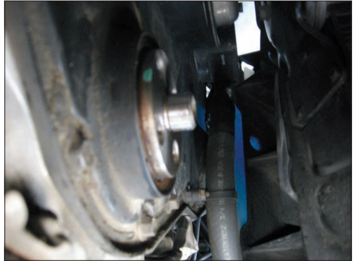
The damper is hub-centric and is aligned on the extension that is machined on the end of the crank. It is important when installing whichever damper you use, to use anti-seize or grease on this hub when fitting the new damper so as not to gall this close-fitting surface when turning the hub for bolt alignment.
