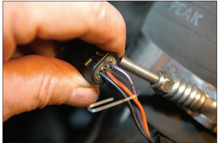
A sharpened paper clip inserted into the center position of the connector.
