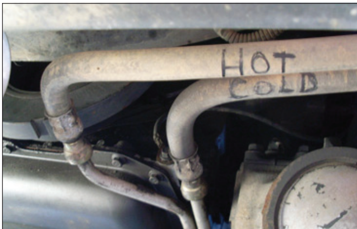
A view of the transmission liner from the front of a Second Generation. Follow the "cold" line back to the transmission cooler and disconnect the line at the junction point. Attach your purge hose to the metal flare at the transmission cooler.
