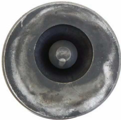
Piston top spray pattern area is visible as gray; incomplete combustion areas are black. This piston is from a vintage '94-'98 12-valve engine. Notice that the piston bowl is offset. The reason for this is that the injectors on the 12-valve engines came into the cylinder head at an angle. On the 24-valve engines ('98.5-'02) and HPCR engines ('03-current) the piston bowl is centered to match-up with the injector that comes into the cylinder head from directly above.
