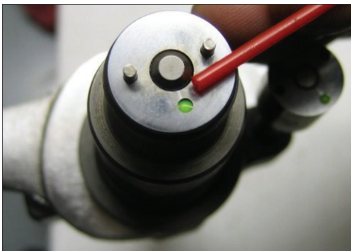
72i15 Cracked injector body.
