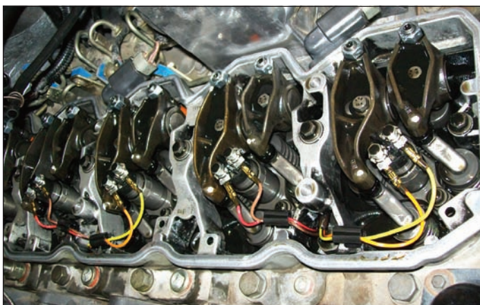
72i6 The rocker lever housing installed on an engine, with injector wiring shown for cylinders 1-3.
