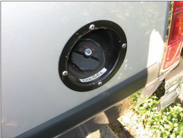
This fuel filler is still available to use in a camper shell or in the truck bed to allow the filling of an auxiliary tank. This one is mounted on a clean First-Gen truck and makes an easy job of filling the spare-tire located tank seen in the previous photo.
