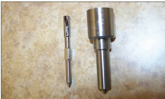
72i12 Pintle with Magic Marker stripe, showing inadequate clearance for the nozzle.
