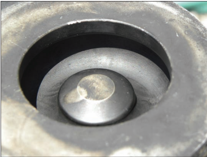
A close-up of the same 12-valve piston showing the piston bowl shape. Note the blunt center top, curved sides.
