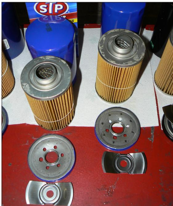
Inspection of the STP filter shows the limited number of holes in the base plate, the stamped metal spring to preload the cartridge, and the minimal number of pleats in the filtration media.
