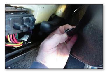
In removing the J-Clips, it helps to put on a pair of rubber gloves to protect your hands. Should your hands slip, the gloves will keep your hands from being cut on sharp metal brackets under the seat.
